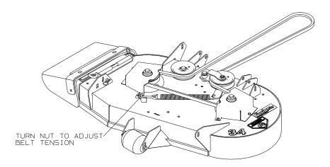
Note: Belt deflection or movement should be approximately 1/4" when measured at mid-point between pulleys. Periodically inspect both belt and idler systems.
